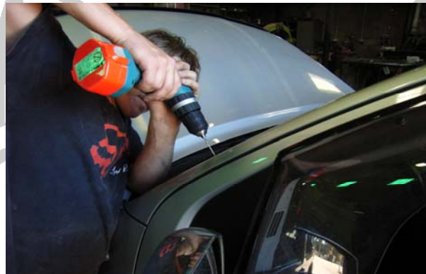
3.26 Drill the 2 x 7mm holes for the "A" pillar position
