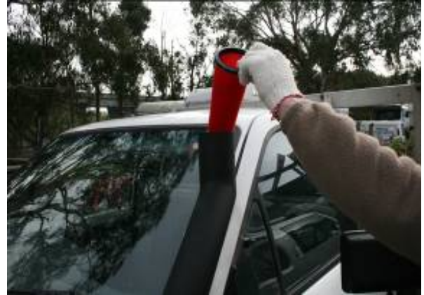
4.2 Install Pre-cleaner filter sock SP065B
