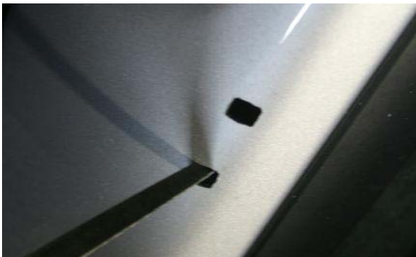
3.27 File the holes with a square file to suit nylon plugs SP026
