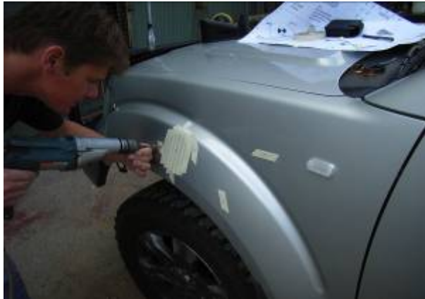
3.16 Pre-drill all holes at 5mm (7 snorkel mounting holes, 1 hole saw hole)
