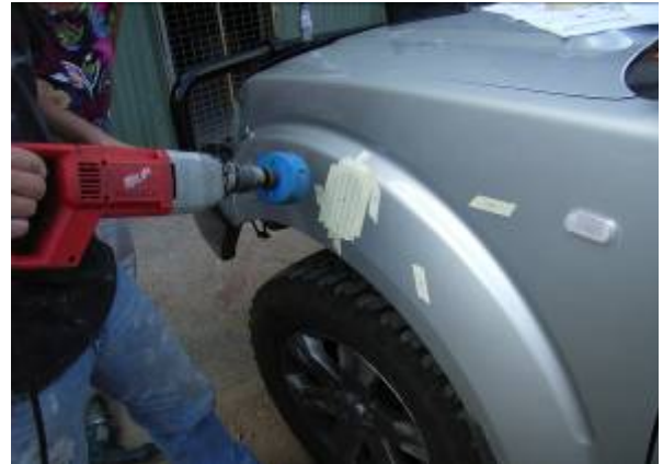
3.17 Using the hole saw, drill at LOW SPEED a 90mm hole
