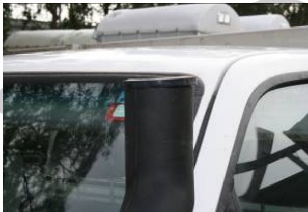
4.3 Air sock should neatly fit into the top of the snorkel body
