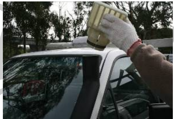
4.4 Re-install the Air ram SP063
