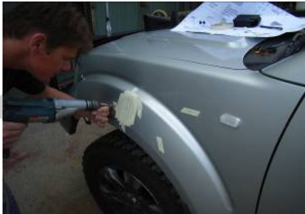
3.18 Drill the 7 snorkel mounting holes at 10mm
