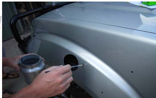
3.28 Paint ALL raw metal surfaces with Zinc rich primer (7 snorkel fixing holes, 1 air intake hole, 2 "A" pillar holes)
