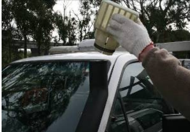
4.1 Remove the Air Ram SP063
