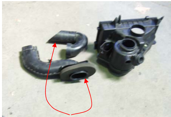
3.30 Remove these parts off the air box and discard them
