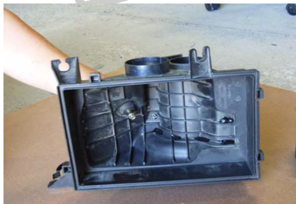
3.35 Re-install the air box in the engine bay but do not bolt it back yet
