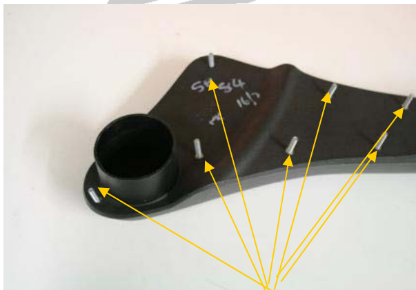
3.20 Screw the 7 studs SP022 with chemical locking compound; at least 20mm must protrude.
