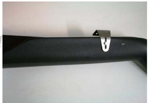
3.21 Fit the "A" pillar bracket SP072 with the washer SP023 and bolt SP024 Do not over tighten fixings to avoid damage to the snorkel
